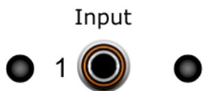
Each input channel has an Input socket and two indicator LEDs. The left-hand LED is red, and will illuminate if this channel currently has the minimum value. The right-hand LED is green, and will illuminate if this channel currently has the maximum value.
