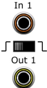
The Input socket accepts any analogue input signal. The threshold for detecting edge transitions is +2.5V.
