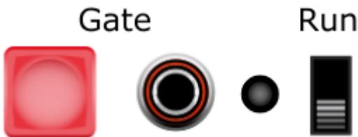
The Integrator will only process its inputs and internal state when in Run mode. When Run is off, the output will remain static. From left to right, the controls are:
