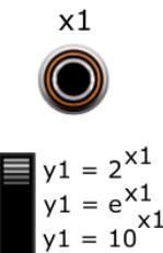
ACE Powers lets you raise a constant value to the power of the X input. There are three selectable constants which are useful within an analogue computer and modular synth environment:
