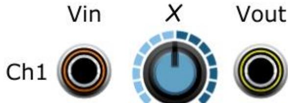
If the Vin socket is disconnected, the channel will operate as a static DC source, with values from -10V to +10V, as set by the X knob.
