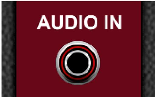
The Audio In socket is where you plug in the signal which you want to attenuate. This is usually an audio source such as an Oscillator or Noise Generator.
