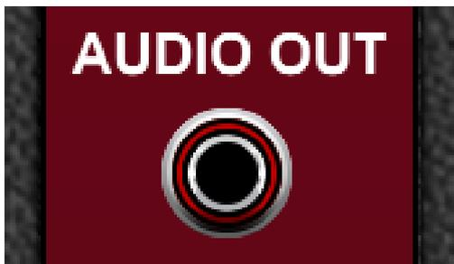
The Audio Out socket is where the module sends its processed Audio In signal, after being attenuated by the Out Level control and the Env In control voltage.
