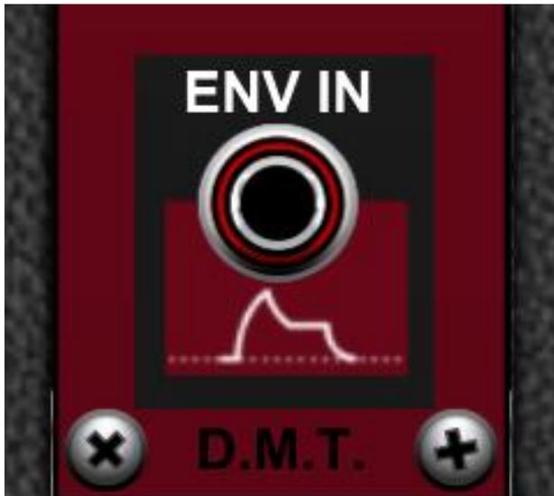
The Env In socket allows you to control the output level with an external voltage source.
