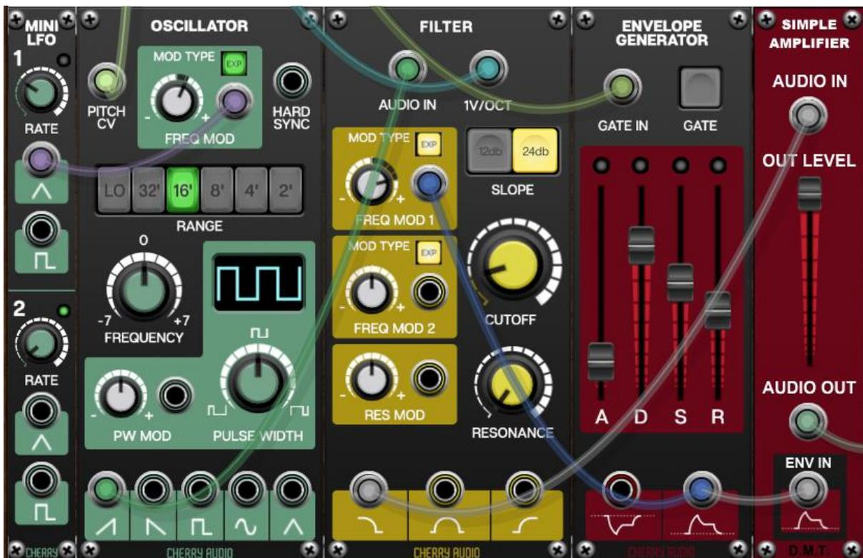
When the envelope voltage is at 0V, the Audio Out will be silent, regardless of the setting of the Out Level slider.
