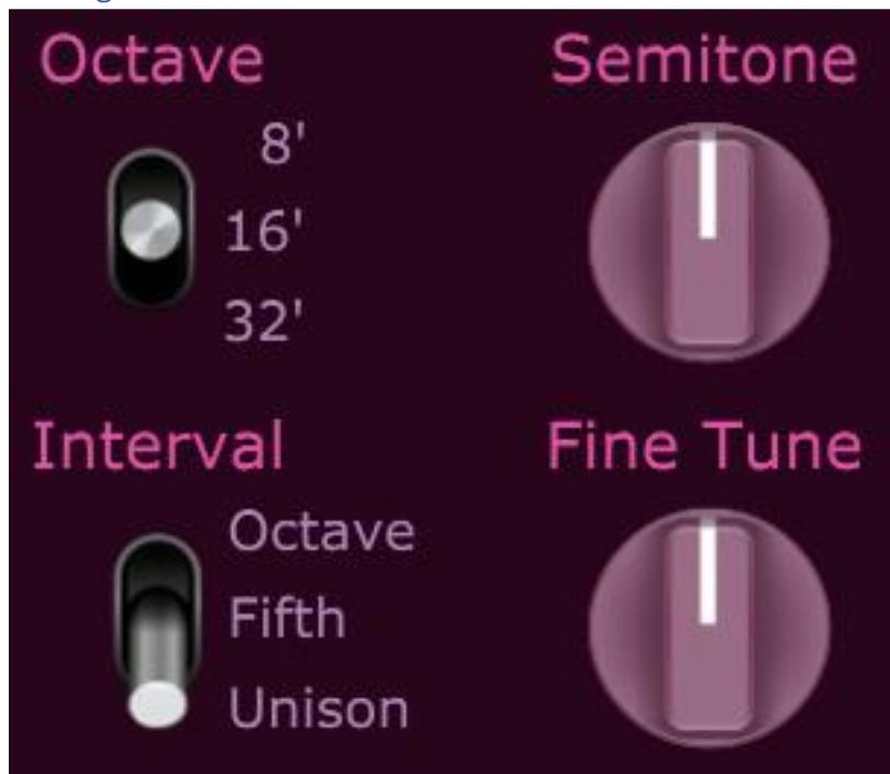
The Octave, Semitone and Fine Tune controls set the basic pitch of both oscillators.
