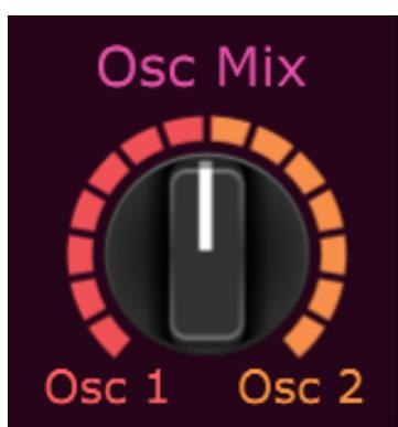
The Oscillator Mix knob adjusts the balance of the two oscillators.
