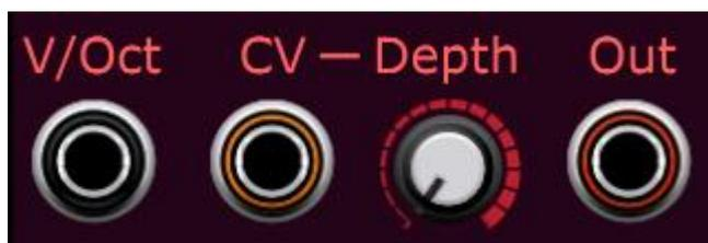
The V/Oct input is normally connected to the keyboard pitch output or sequencer output. Any volts-per-octave source can be used though, even audio signals.
