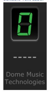
Below the seven-segment LED indicator, there is an editable text field which allows you to label the drawbar. This can be used to identify its purpose - for example "8" to indicate the "8 foot" rank. The label initially displays five dashes "-----", but can be edited by double-clicking the mouse over that part of the panel:
