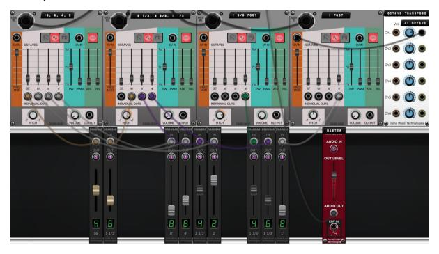
The output of each drawbar channel can be used independently, but it is often convenient to use the Voltage Modular 'Cable Buses' to combine the outputs into one common signal, similar to how a standard mixing desk works. In the image above, Cable Bus 1 (purple) is fed to the input of a <a href="Simple Amplifier">Simple Amplifier</a>, acting as a master volume control.
