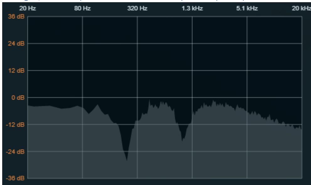
5 Stages, Normal (Two notches with low-pass response)
