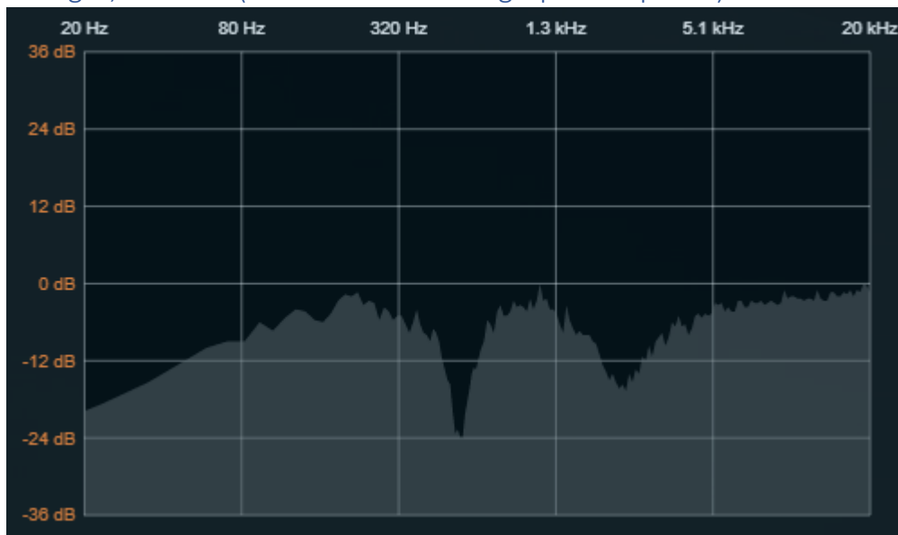
5 Stages, Inverted (Two notches with high-pass response)
