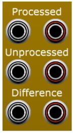
The 'Processed' output is the signal which has been sent through the dithering and quantisation steps.
