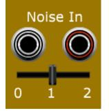
Before quantisation is applied, you have the option to add dither noise to the input signal. The TPDF Noise Module is the ideal source for dither noise, but any input signal may be used instead. The attenuation slider allows you to set the dither level from 0 (fully left) to 2 Least Significant Bits (fully right). As the main bit depth control is increased in value, the relative amplitude of the dither noise will decrease automatically.
