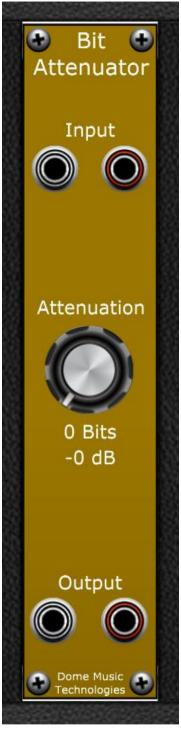
The Bit Depth Attenuator Module takes a stereo input and attenuates it from 0dB to -144dB in 6dB steps.
