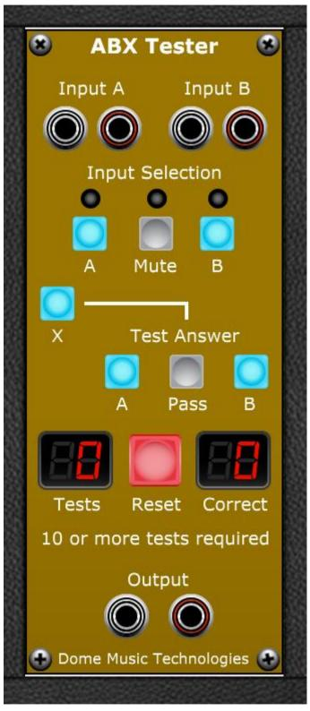
The ABX Tester Module allows you to switch between two stereo inputs to determine if you can perceive any difference between them. For example, you could use the Processed and Unprocessed outputs of the Bit Reducer Module, and see if you can tell any difference between a double-precision floating point signal and one which has been quantised to 16 bits.
