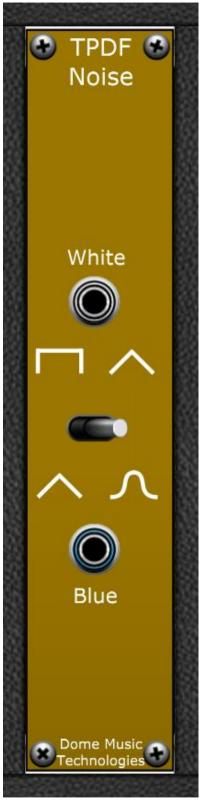
The TPDF Noise Module provides sources of white and blue noise with selectable Probability Density Functions (PDFs). It was designed to be used as a source of Triangular Probability Density Function white noise for dithering purposes in the Bit Reducer Module. Uncorrelated stereo TPDF noise can be generated by running two instances of the module in parallel – one providing noise for the left channel and one for the right channel.
