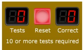
The Test Results Panel keeps track of the number of tests you have run and the number of correct answers you entered. The Tests and Correct seven-segment LED counter displays can record up to 99 each. The red Reset button in the middle resets both the Tests and Correct counts to zero and returns the module to Monitor Mode.
