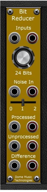
The Bit Reducer Module quantises the stereo input signal in steps from 1-bit to 24-bits. There is a dither noise input and attenuator. Finally, there are three outputs which let you compare the original signal against the quantised one.
