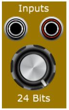
The Bit Reducer Module has stereo inputs and two independent (left / white and right / red) processing channels. It can also be used as a monoaural effect by selecting one channel and ignoring the other.
