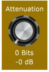
The Bit Depth Attenuator Module can attenuate the input signal from 0dB down to -144dB in 6dB steps. The Attenuation knob is calibrated in integer bits (from 0 to 24). Each bit of attenuation represents a halving of signal amplitude (equivalent to a gain of -6dB).
