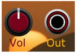
Volume can be adjusted from 0 (7 o'clock) through 100% (12 o'clock) and up to a maximum of 200% (5 o'clock). As mentioned previously, the volume level drops automatically when the polyphony count (Number of Voices) is increased.
