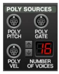
The "Number of Voices" setting allows you to adjust the polyphony count of Micro Stringer. As the polyphony count increases, the overall output volume level is decreased automatically. This helps to prevent overload and distortion in downstream modules.
