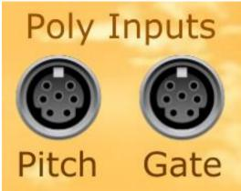
The Poly Inputs section provides you with Poly Input Jacks for Pitch and Gate signals. If cables are not connected to these inputs, then they are 'normalled' to the Poly Pitch and Poly Gate signals on Voltage Modular's IO Panel.
