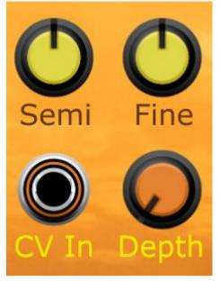
As well as the octave selector switch, Micro Stringer is equipped with a Semitone Knob and a Fine Tune knob. The Semitone Knob allows you to transpose the tuning up to +/- 12 semitones, in semitone steps. The Fine Tune Knob allows you to make fine pitch adjustments up to +/- 1 semitone.
