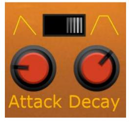
Micro Stringer has an independent volume envelope generator for each voice. This avoids the abrupt 'voice stealing' behaviour of some older string machine designs.
