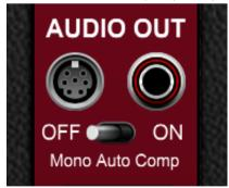
The Poly Simple Amplifier has both Poly and Mono (mixed) outputs available. Use the Poly output if you want to keep each voice's signal separate, for further processing. The Mono (mixed) output is useful if the Poly Simple Amplifier is the final module in your polyphonic patch.
