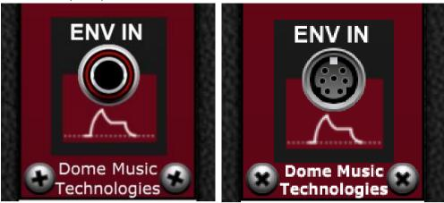
The Env In socket allows you to control the output level with an external voltage source.
