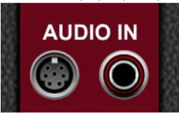
The Poly Simple Amplifier has two Audio In sockets: Poly and Mono.
