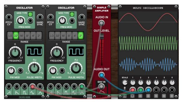
In both versions of the Simple Amplifier, the ENV IN and AUDIO IN sockets can be used interchangeably (when both are used simultaneously). i.e. You can plug your envelope generator into the AUDIO IN and your audio signal into the ENV IN, and get exactly the same result at the output. However, if you are using it as a simple attenuator, then you MUST plug the audio signal into the AUDIO IN socket, otherwise you will get silence at the output.
