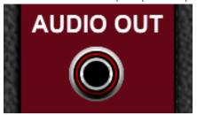
The Audio Out socket is where the module sends its processed Audio In signal, after being attenuated by the Out Level slider control and the Env In control voltage.
